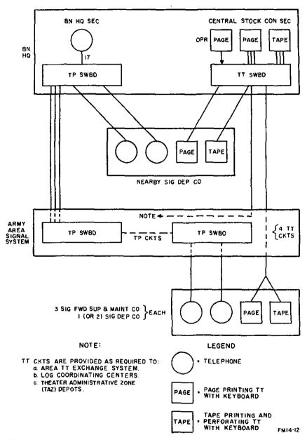
Figure 3. Type battalion telephone and teletypewriter communication system.
